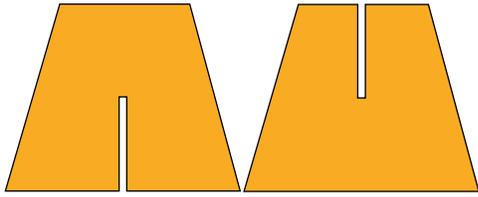
Cut slots the same width as the thickness of the fin stock.
