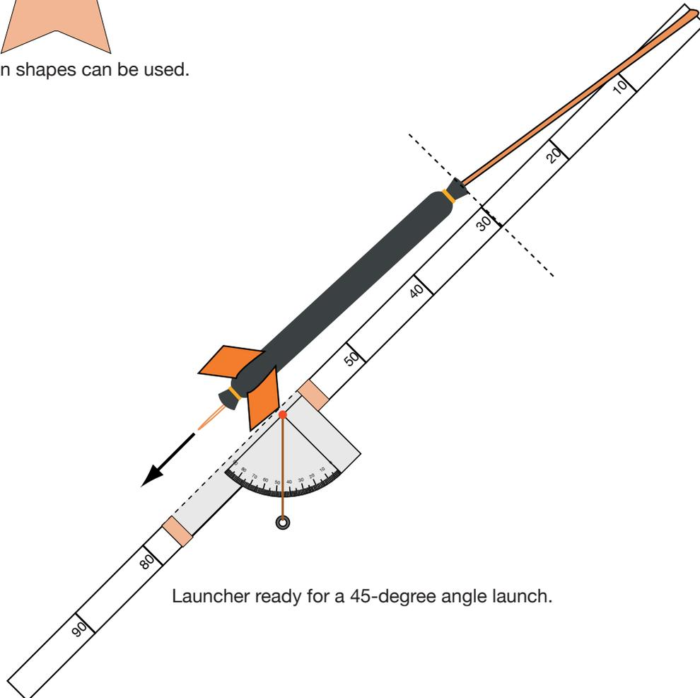
Launcher ready for a 45-degree angle launch.
